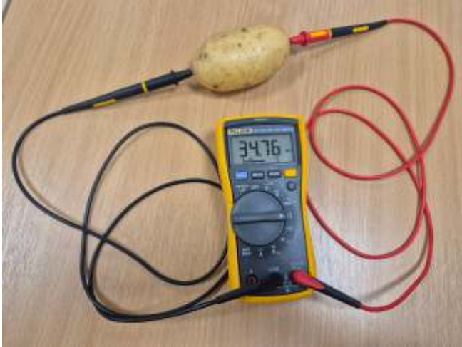
Figure 3 - Potato, showing resistance of 3.5 \times 10^4 \Omega , within Type C FIBC object recognition window.
