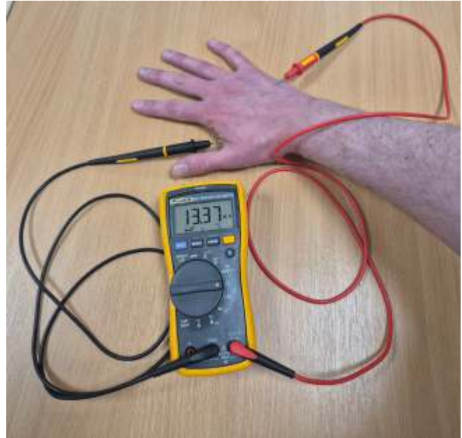
Figure 2 - Human hand, showing resistance of 1.3 \times 10^7 \Omega , within Type C FIBC object recognition window.
