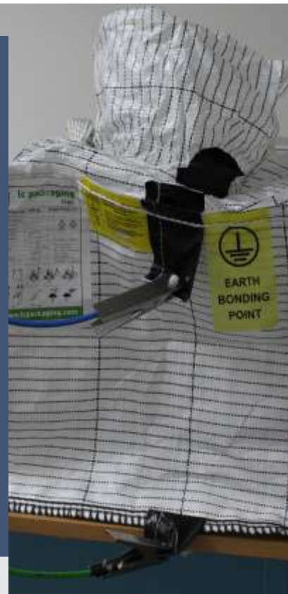
Figure 1 - An example of a safe connection to an earthing point.
