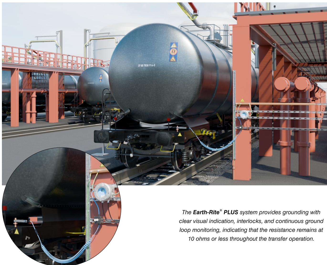
*The **Earth-Rite® PLUS** system provides grounding with clear visual indication, interlocks, and continuous ground loop monitoring, indicating that the resistance remains at 10 ohms or less throughout the transfer operation.*
