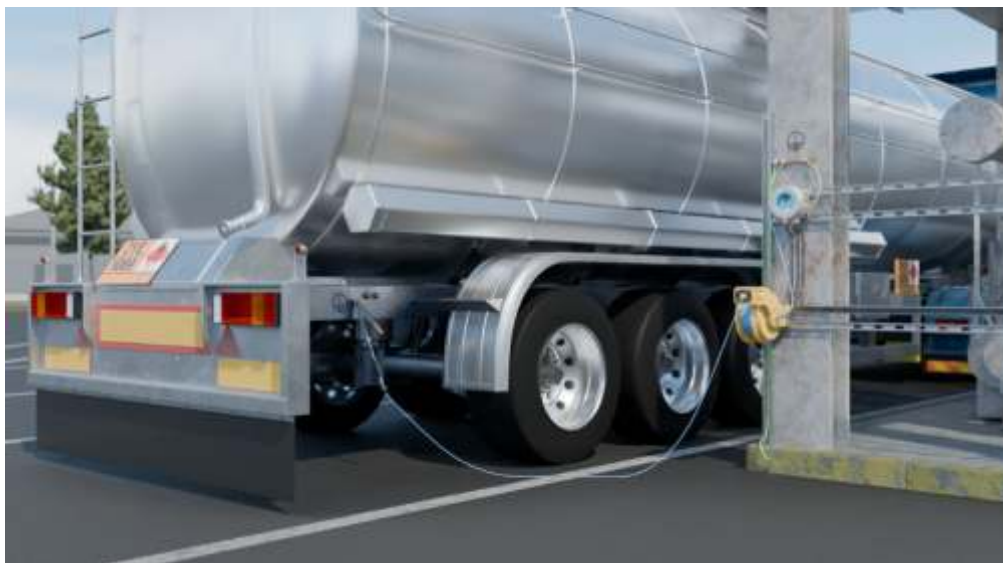
The Earth-Rite® RTR system provides grounding with clear visual indication, interlocks, and continuous ground loop monitoring, indicating that the resistance remains at 10 ohms or less throughout the transfer operation.
