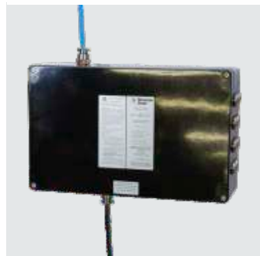
The Earth-Rite MULTIPOINT II's 230 V/110 V AC power supply unit houses eleven (11) SP/DT volt free contacts. 8 of these interface with each monitored grounding channel, 2 provide the grouped channel function and 1 relay provides the fail-safe redundancy output function. The power supply can be installed in Zone 2/21 and Class I, Div.2, Class II, Div.1, Class III, Div.1 areas. The power supply can be housed in GRP or stainless steel enclosures.
