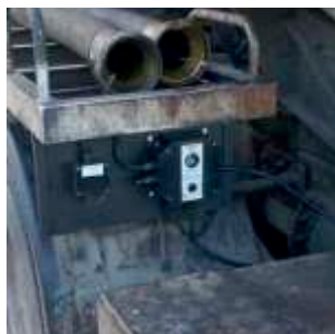
The Earth-Rite II MGV static grounding system can be mounted on vacuum trucks and tank trucks.
