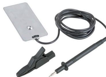
The extension assembly (OGC/EXT) consists of an alligator clip, a test probe and stainless steel plate. It is ideal for testing equipment that does not have a large enough surface to connect to with the OhmGuard clamp. The person performing the test simply connects the OhmGuard's clamp contacts to the plate and then connects the probe or alligator clip to the equipment being tested.
