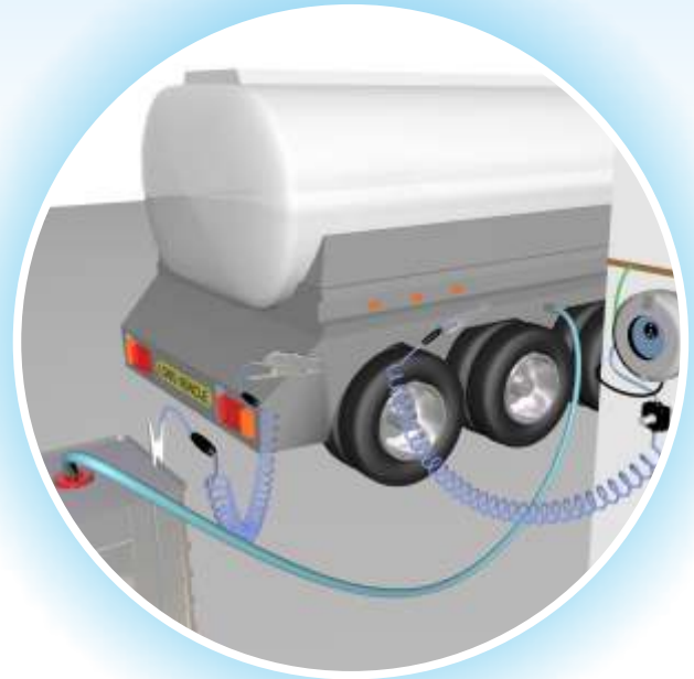
Example of grounding truck bonded to IBC
